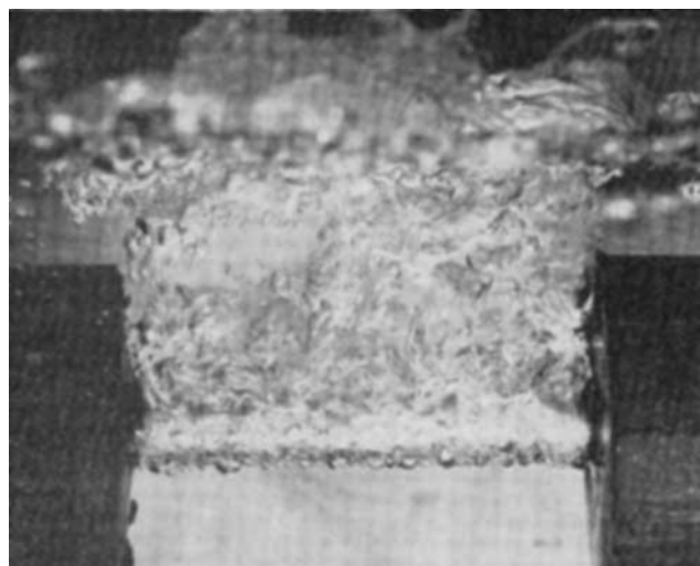
Fig. 4. Normal nucleate boiling of isopropanol \Delta T_o = 60^\circ\text{F} .
